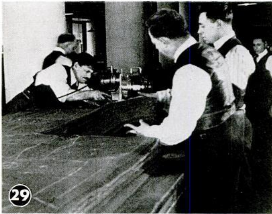
Making 14,000,000 uniforms for Army is speeded by this electric cutter which slashes into bolts of khaki, cuts 60 uniforms at once.
